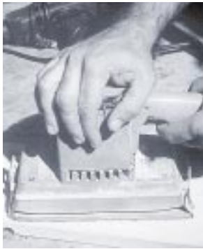
Hand-arm vibration— vibrating sander
