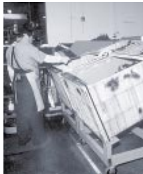
Tilted container with step for easier access
