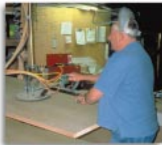
▲ Lift-assist device eliminates manual handling
