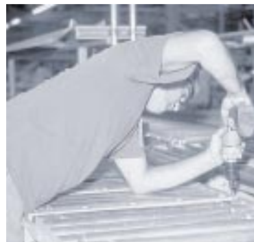
Lack of access or clearance—bending and awkward upper body posture
